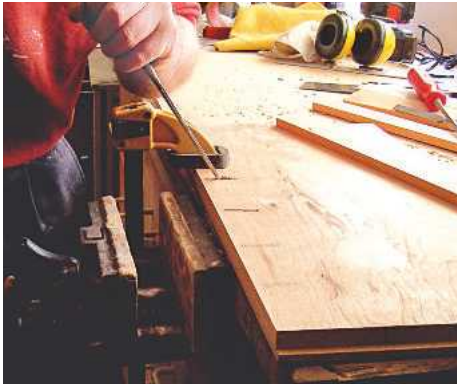
▲ Pic.1 Mortising the sides of the cabinet...
